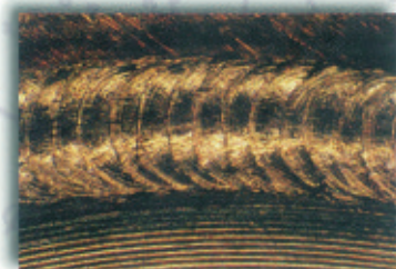
Extreme close-up of weld.
